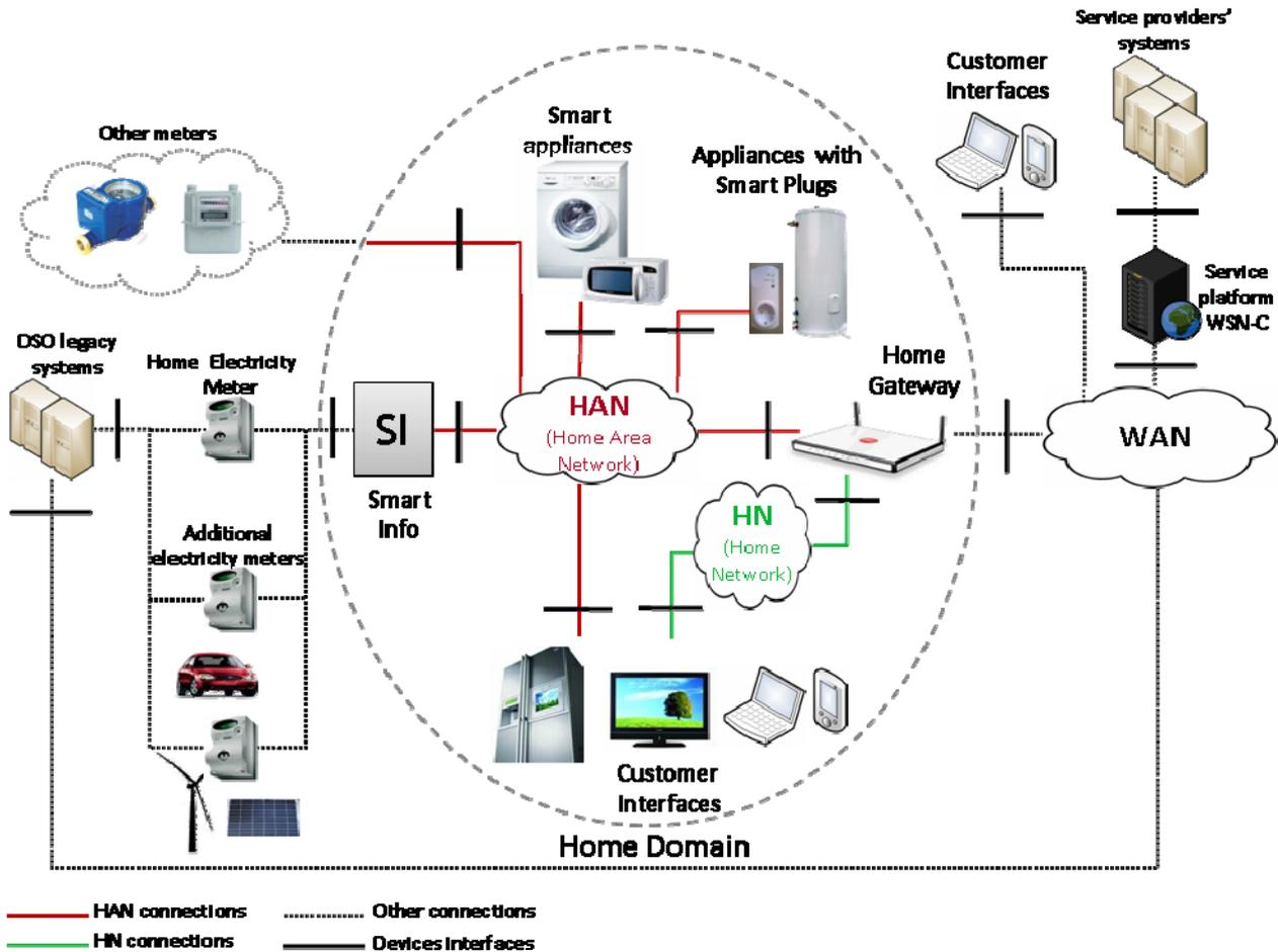
The part inside the dotted area (that includes both the HAN and the HN) is user's Home Domain, where all the actors (Smart Appliances, Home Gateway, Smart Info and Customer Interfaces) can cooperate through some communication mechanism. All the depicted interfaces are logical ones and could be implemented through one or more communication technologies.
